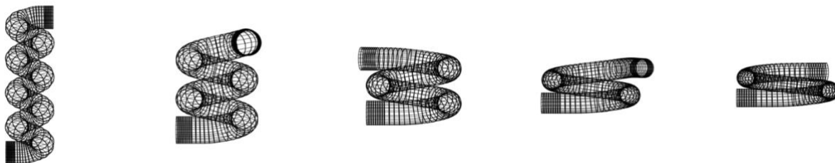
Figure 2: The effect of coil radius for a helical coil tube with a fixed length.
